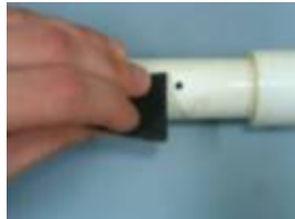
2. Clean/roughen area with 150 grit sandpaper.
